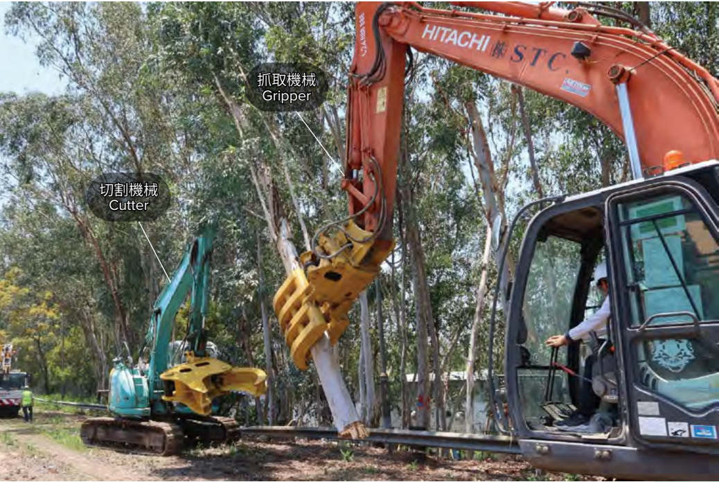
試驗以抓取和切割機械移除樹木 Trials of removal by gripping & cutting machinery
