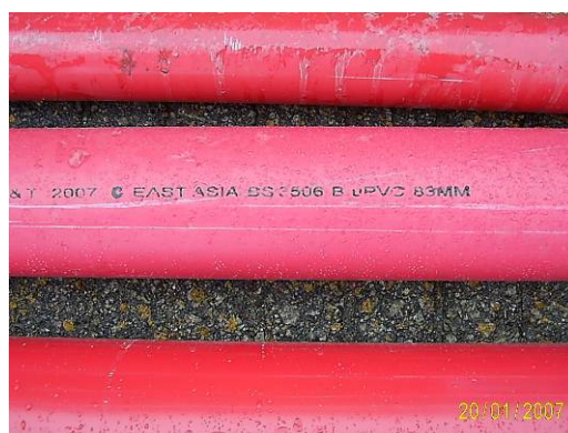
Photo No.5 (PVC Duct : Diameter 56mm to 107mm)
