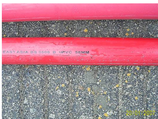
Photo No.5 (PVC Duct : Diameter 56mm to 107mm)
