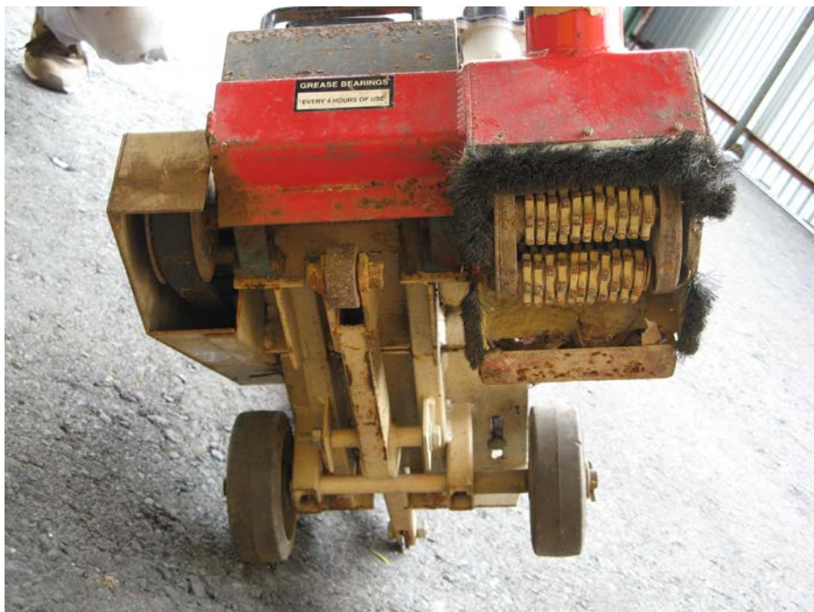
Plate No. 18 Type 2 Grinding Machine (in Pure Scarifying Motion)
