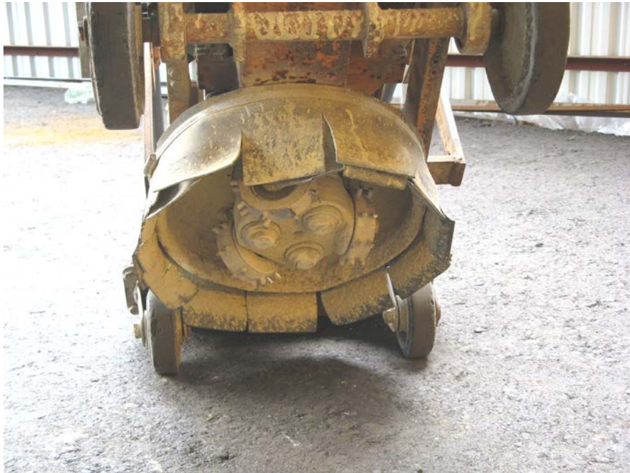
Plate No. 17 Type 1 Grinding Machine (in Circumgyrate Centrifugal Motion)
