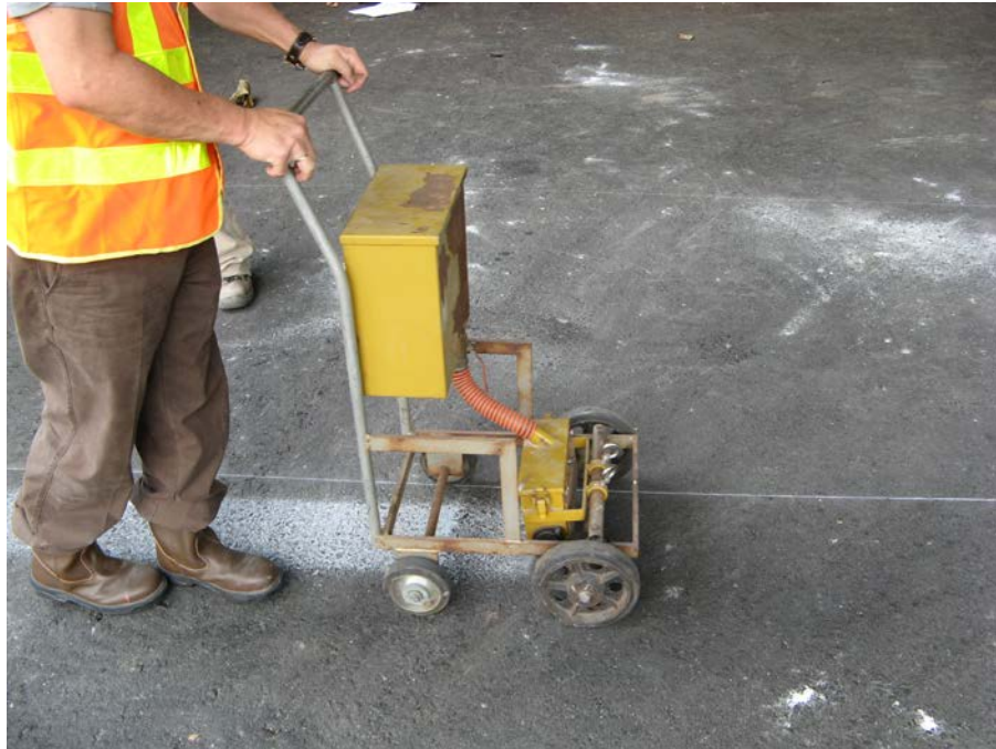
Plate No. 15 Hand Push Trolley for the Dispense of Glass Beads
