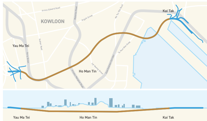
Alignment of the Central Kowloon Route
