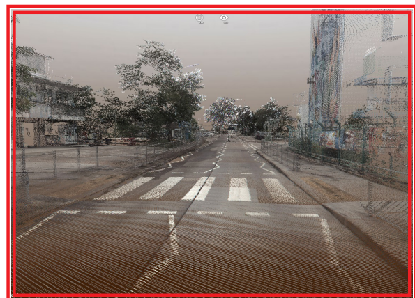
The photo-textured 3D point cloud in MLSI survey
