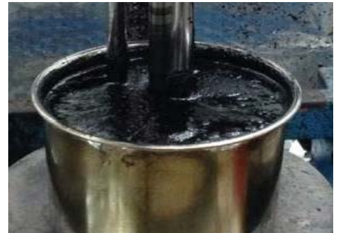
Crumb Rubber Modified Bitumen in laboratory
