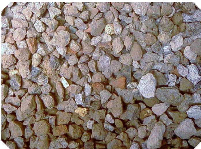
Recycled Aggregates Used as Sub-base Materials
