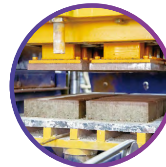
Precast concrete paving units with recycled plastics
