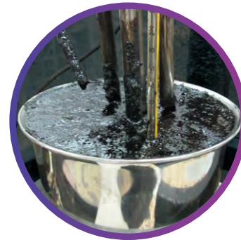
Crumb rubber modified bitumen in laboratory
