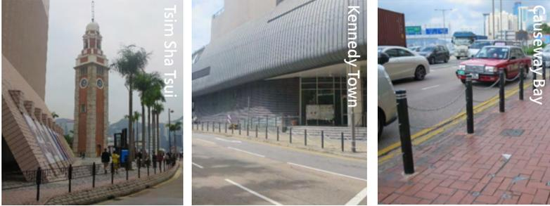
The pedestrian railings in the tourist spots are upgraded by replacing obsolete/ redundant railings, replacing old ones by new prototype, and adopting half panels or bollards at suitable locations to provide a more open view.
