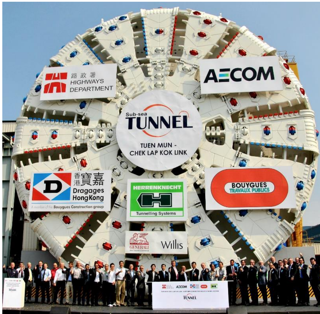
17.6-metre Diameter TBM
