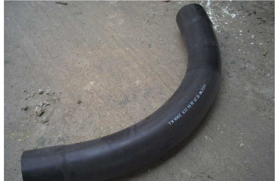
Photo No. 4 (PVC Bend Duct : Diameter - 107mm) Buried at Depth : 450mm
