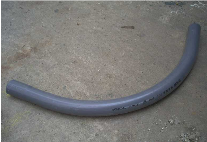
Photo No. 3 (PVC Bend Duct : Diameter 56mm) Buried at Depth : 450mm
