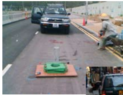
Drainability Test - for measuring hydraulic conductivity
