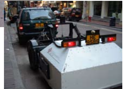
Close Proximity Method (CPX) - for measuring road/tyre noise level
