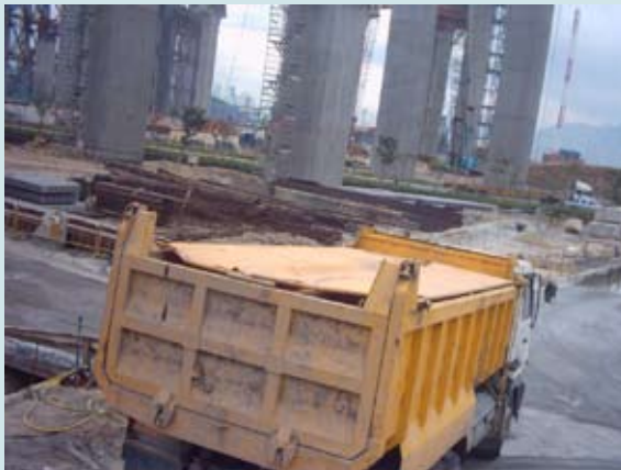
Dump truck fitted with automatic covers
